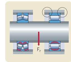
By avoiding induced axial loads, both bearings share the radial load evenly.
